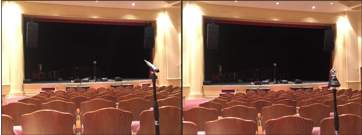
Figure 8 – Room Impulse Response Measurement Using M30BX and H3-VR at a Same Location
