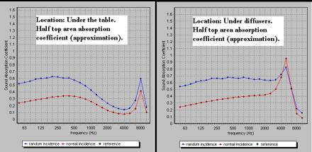
Notes: There are four to eight different bass traps in the studio. Using four basic designs, various cavity depth and various fiberglass density, the bass traps are approximated to provide higher absorption coefficient values compared to the ones predicted by computer. This is confirmed subjectively by comparing floor tom sound reproduction before and after bass trap installation.
