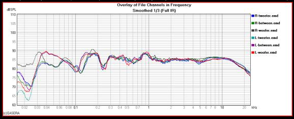
Each left and right measurements are averaged and the result is shown below (1/3 and 1 octave smoothing).
