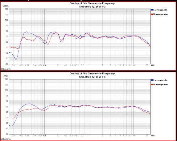
Tannoy Reveal6P operating range is 30Hz – 18000Hz (+3dB, -4dB) in this room (1 octave smoothing).
