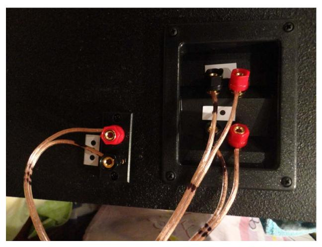
Each cable is marked by dots (one, two or three) and each pair has one end that is marked by a black marker. The dot on the cable corresponds to the dot on the sticker near the terminal. The black marker at the end of the cable corresponds to the negative (black terminal) input.
