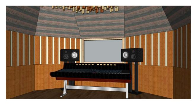
Above picture shows the <u>preferred</u> setup. Woofers are located "inside" and loudspeaker is mounted horizontally. This box position is the default position for E-33A-100701.
