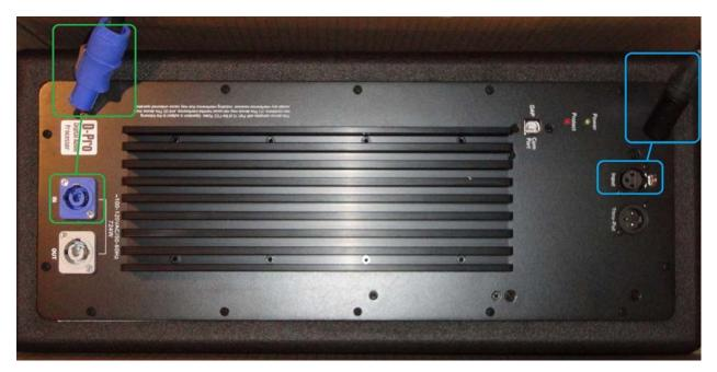
Please make sure to rotate the power cable to properly turn on the amplifier. A click will be heard when the power cable is properly attached.
