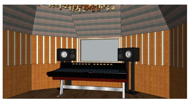
Above picture shows another variation of the horizontal position. Placing woofer "outside" may result in slightly narrower stereo image.
