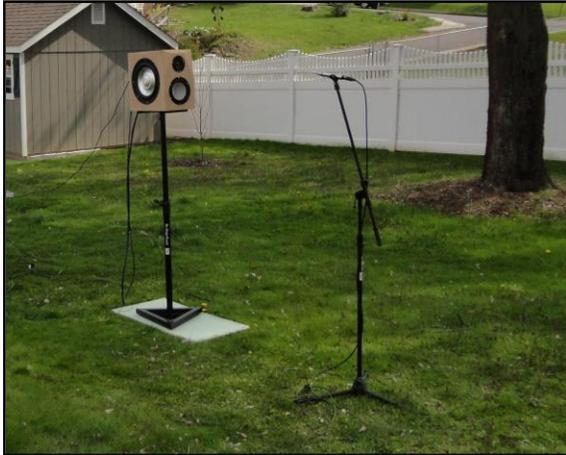
This measurement condition will include a ground reflection. The frequency response usefulness will be limited from the first reflection (usually from floor). The impulse response shown in the photo on the left can be seen below.
