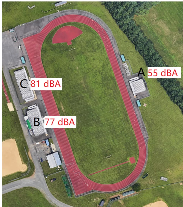
Figure 6 - Maximum level with pink noise turned on, A-weighted and slow response, at three locations
