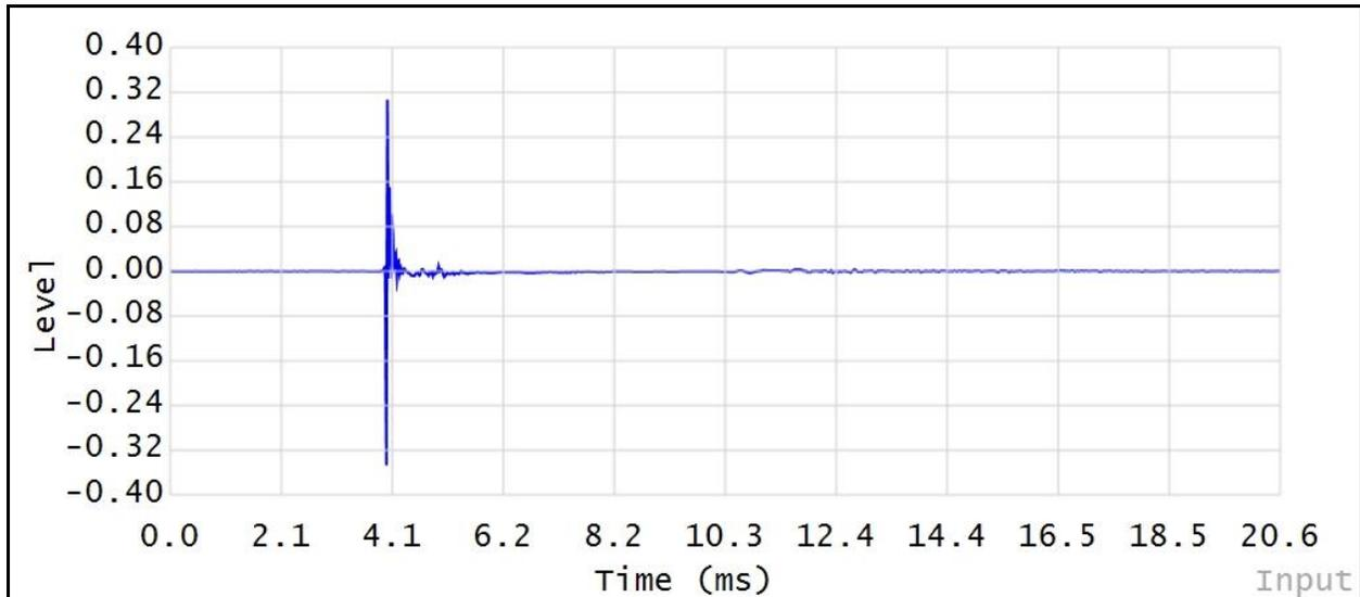
The direct sound arrival is approximately at 3.9ms and reflections can be noted at around 11ms. First, we like to move the impulse response cyclically to the beginning, so the very early energy arrival is located at zero. In this sample, the first impulse response energy arrival comes at 4 samples prior to the peak of the impulse response.
