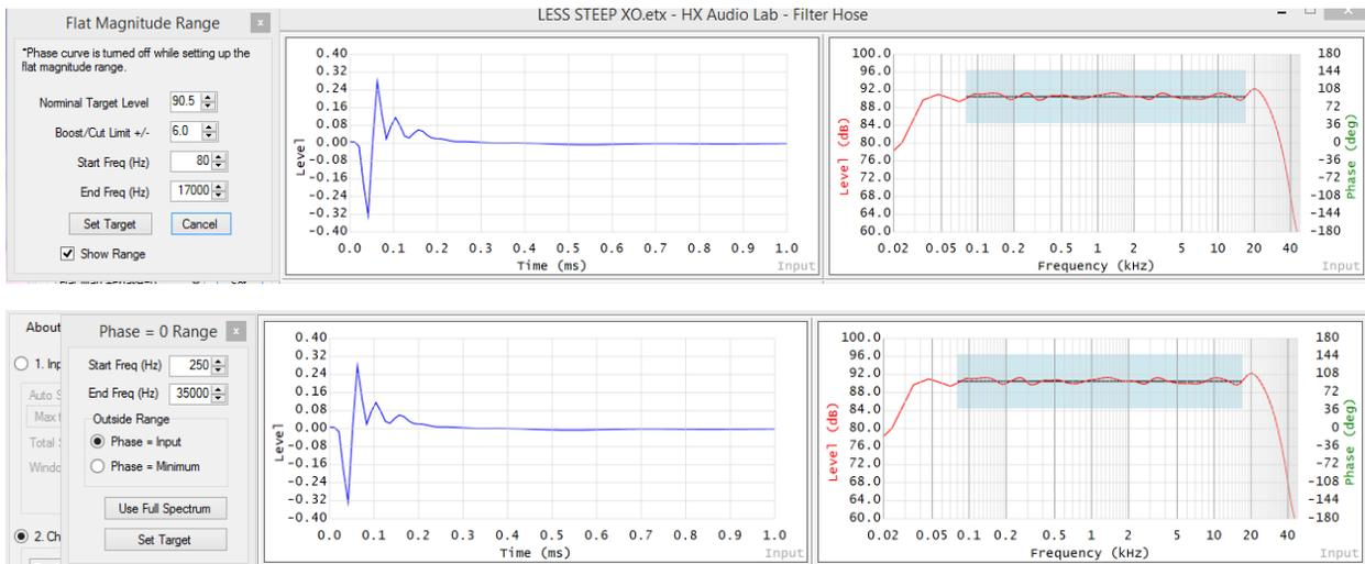
In this example, the magnitude will be flattened from 80Hz to 17000Hz and the phase will be flattened from 250Hz to 35000Hz.
